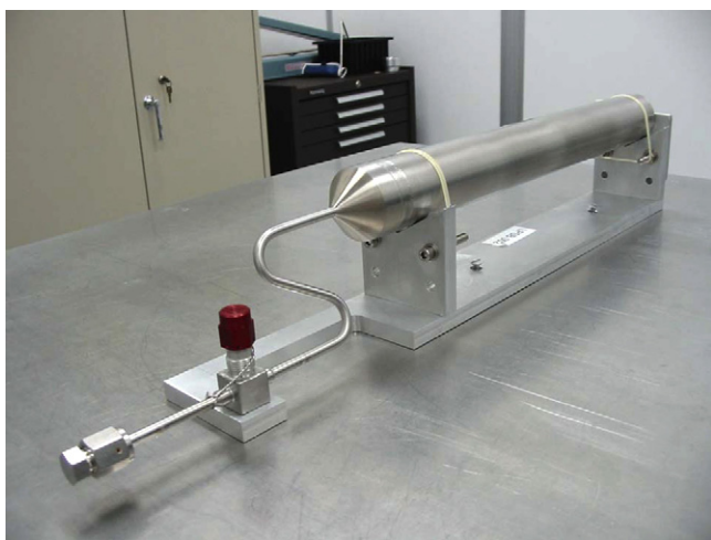
Fig. 1. Photograph of a low-pressure storage bed (LPSB) from the JPL Planck sorption cryocooler project that can be modified (i.e., greatly enlarged) to store sufficient quantities hydrogen to operate 1–5 kW size PEM fuel cell power systems.
